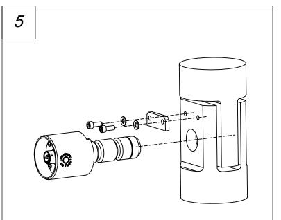
Assemble keeper plate, washers, screws, and pin into the supporting structure.
