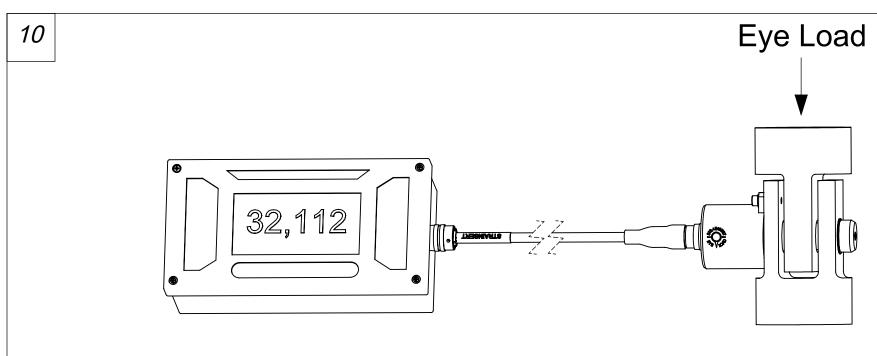
Follow the instrument set-up instructions. Null out preload. In-place calibration check recommended. Refer to the Strainsert Calibration Certificate.
