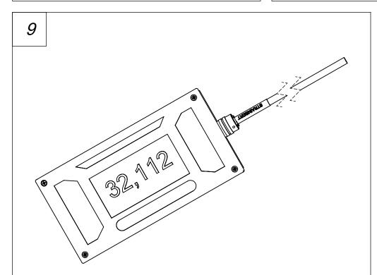
Attach the cable to the instrumentation. Intrumentation can vary.
