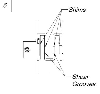
Add Shims if required to center the shear grooves in the clevis/eye.
