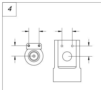
Locate hole position for keeper plate. Tap holes into your supporting structure for screws.
