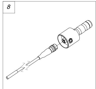
Plug cable into the pin connector.
